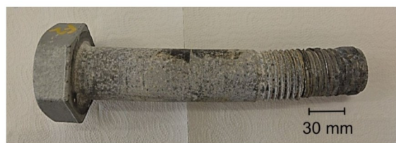
Influence of Corrosion on Fatigue of the Fastening Bolts
